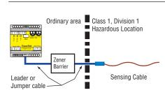
If protected by an agency approved zener barrier, TraceTek sensors in Class I, Division 1, Groups A, B, C, D Hazardous Locations (Zones 0 and 1 in Europe). Contact Tyco Thermal Controls to select proper zener barrier.
