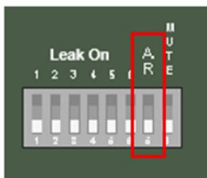
**Important!** Alarm history is not retrievable from the Eco-6+, auto reset should only be enabled if the panel is connected to a BMS or master panel that can record alarm events.
