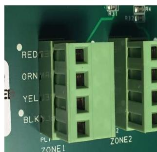
**NOTE: Do not connect more than one sensing circuit into each zone. Doing so will cause malfunction in the cable break checking system and may prevent the panel from detecting cable faults and leaks.**
