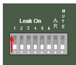
To enable a zone, simply move the dipswitch into the on (up) position
