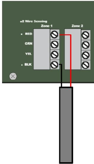
1) Eco-Leak 2 Core leader cable is connected as shown. The connectors are colour coded and for two core you will need to utilise black and red.
