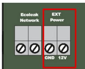
The Eco-6+ has a 12Vdc output for the powering of accessories such as AT-OPSENS (max 6) or the AT-RAP. The maximum load available from this is 500mA. Exceeding this may cause damage to the panel.
