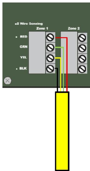
1) TraceTek 4 Core jumper cable is connected as shown. The connectors are colour coded, yellow, black, green and red.
