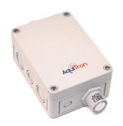
Exchangeable sensor unit including digital value processing, temperature compensation and self-monitoring the ambient air. The AT-MC Pellistor sensor houses a module with controller, analogue output and power supply. The AT-MC calculates a linear 4–20 mA (or 2–10 V) signal out of the measurement signal and stores all relevant measured values and data of the sensor element.
