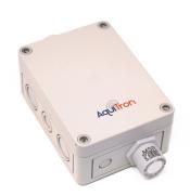
Exchangeable sensor unit including digital value processing, temperature compensation and self-monitoring the ambient air. The sensor houses a module with a terminal for the analogue output. The AT-MC calculates a linear 4–20 mA (or 2–10 V) signal out of the measurement signal and stores all relevant measured values and data of the sensor element.
