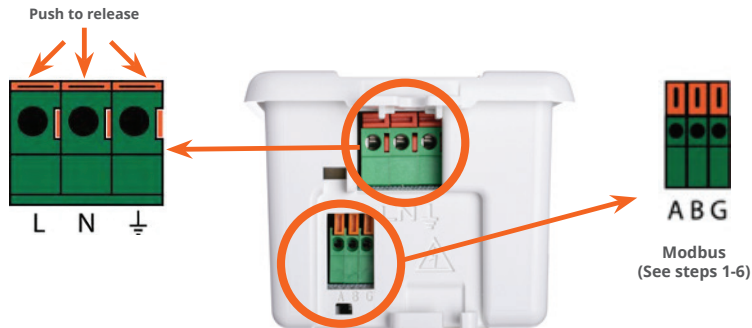
Figure 6. Wiring Power & Modbus
