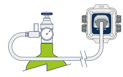
2. If using a variable flow regulator, adjust the gas flow to approximately 0.3 L/min.
