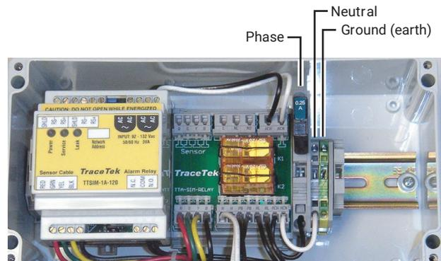
Figure 3. Power connections
