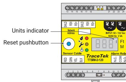
Figure 11. RESET pushbutton and units indicator locations
