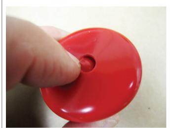
Push the TraceTek cable through the hole. You may need to bend the end cap to open the hole enough for the cable end to pass through.
