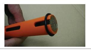
• Insert TT-FFS into clear mesh tube. When fully inserted, o-ring will be centered in tube.
