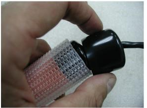
**Note:** The EEC should be inspected monthly for blockage. If the mesh tube becomes contaminated with dirt or debris, it could prevent a leak from being detected rapidly. To clean the EEC, remove the cap, carefully remove the TT-FFS, and wash the EEC in water or IPA (Do not remove screen!). TT-FFS cleaning (if necessary) is a separate operation, please refer to TT-FFS Care and Cleaning Instructions (H58307).
