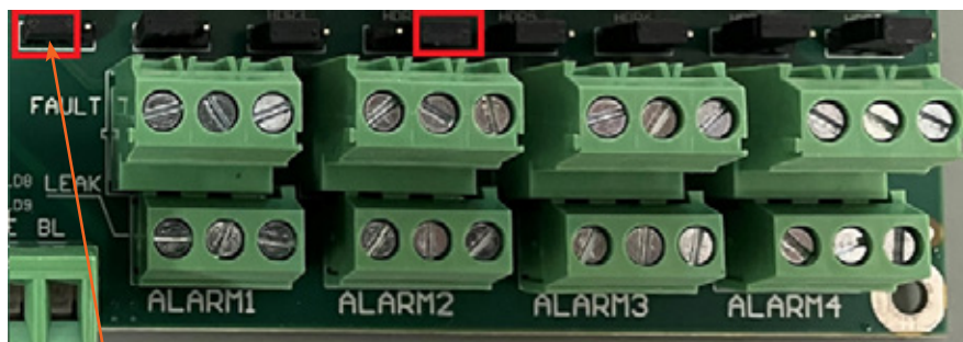
FAULT Relay N/O position Jumper in LEFT position (Default)
