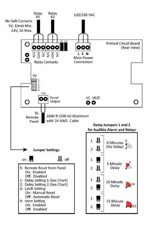
NOTE: The maximum wire size into terminal blocks is 16 AWG.
