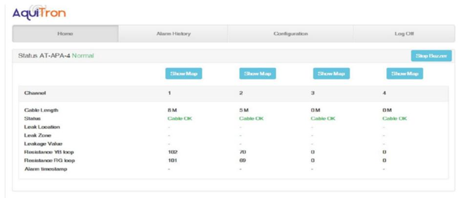
The screenshot shows the Aquitron web interface. At the top, there are navigation tabs: Home, Alarm History, Configuration, and Log Off. Below the tabs, the status is "Status AT-APA-4 Normal" with a "Stop Alarm" button. There are four "Show Map" buttons above a table. The table has columns for Channel 1, 2, 3, and 4. The rows include Cable Length, Status, Leak Location, Leak Zone, Leakage Value, Resistance YB loop, Resistance FG loop, and Alarm timestamp.
