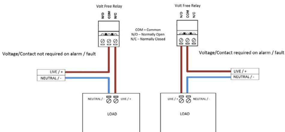
Please ensure that the load does not exceed the ratings of the volt free relay. This is stated in the relevant product's data sheet / installation instructions.
