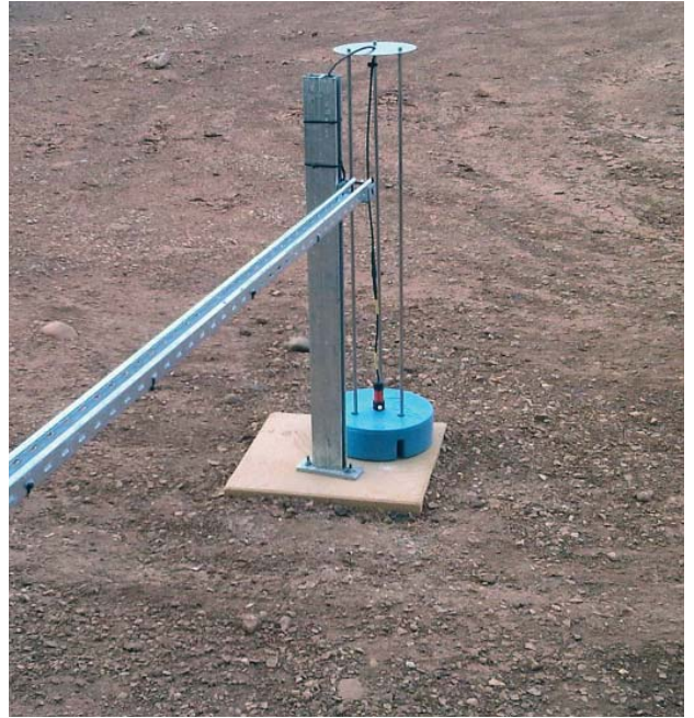
TraceTek Fast Fuel Sensor (TT-FFS) attached to a float assembly with the bund.
