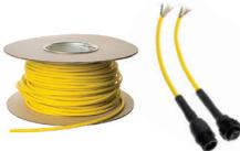
Jumper cable, (yellow), LSZH rated on bulk reels for directly connecting into the PROBE-TS or for connection to the modular sensing cable after fitting the necessary connectors. Male and female connectors with a 250mm tail are available separately and can be spliced on to the bulk jumper cable with a splice kit TT-JSK-HS18 (kit contains parts for 5 cable joints)
