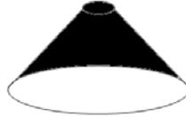
Collectors are typically used when detecting ammonia where the gas being detected is lighter than air. Collectors are typically positioned at working height above potential leak sources and trap pockets of air which may contain ammonia and funnel them into the sampling pipe work. End of line filters are fitted in the centre of the collector to protect the sampling pipe work. The collector can be secured to the underside of steel beams or hung from threaded rods as required.
