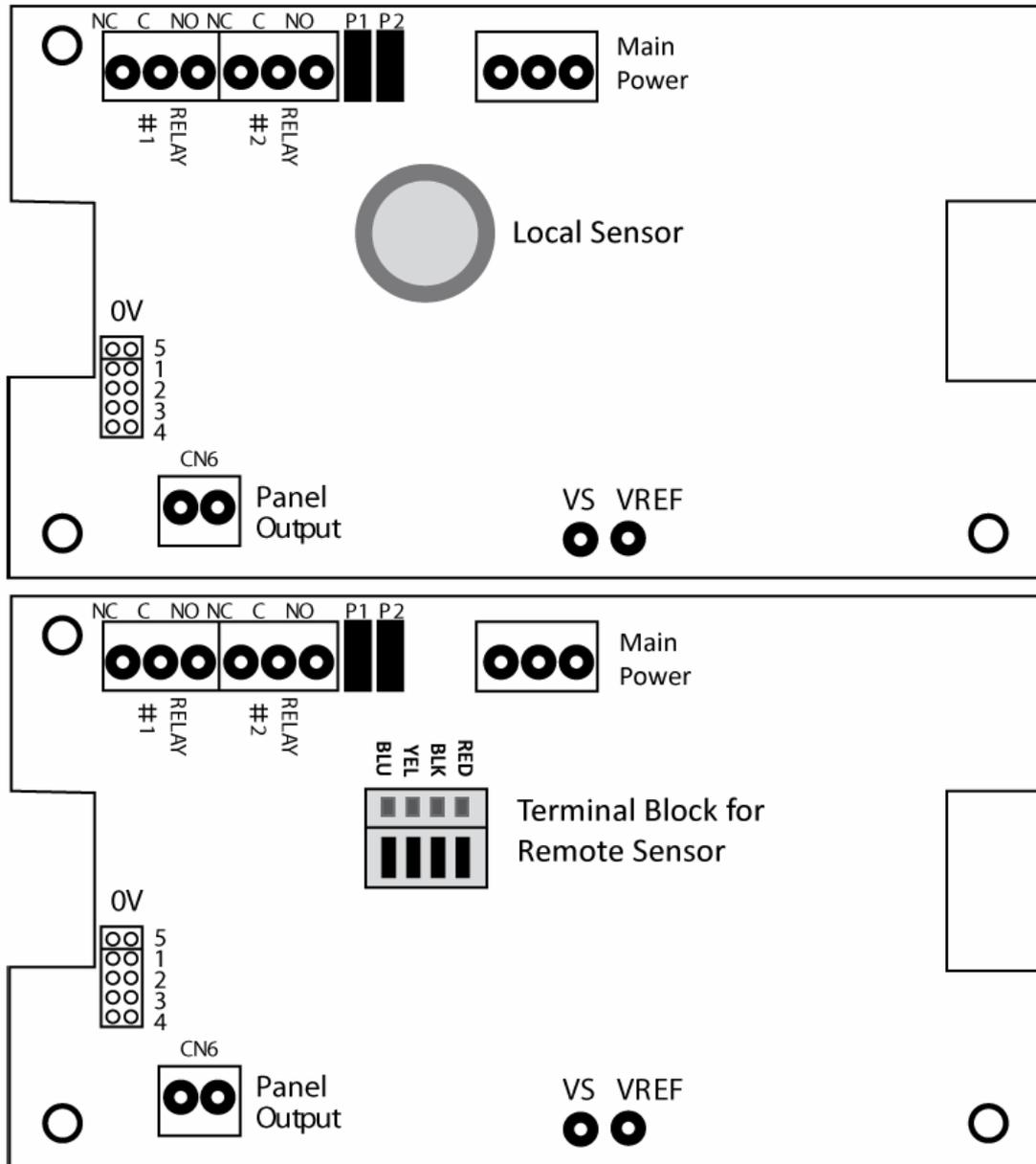
**NOTE:** For remote sensor configurations, the sensor is mounted on a small remote sensor board that connects to the AT-G-SENSE's main PCB via a 4-wire connecting cable.
