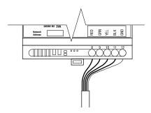
Figure 6. Sensing Cable Connections
