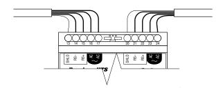
Figure 4. Power and Telemetry Connections
