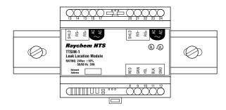
Figure 1. DIN Rail Mount
