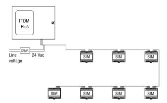
Figure 3. Power Supply to SIM units
