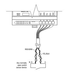
Figure 7 Switch Type Sensor
