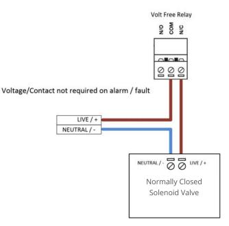
Please ensure that the load does not exceed the ratings of the volt free relay. This is stated in the relevant product's data sheet / installation instructions.
