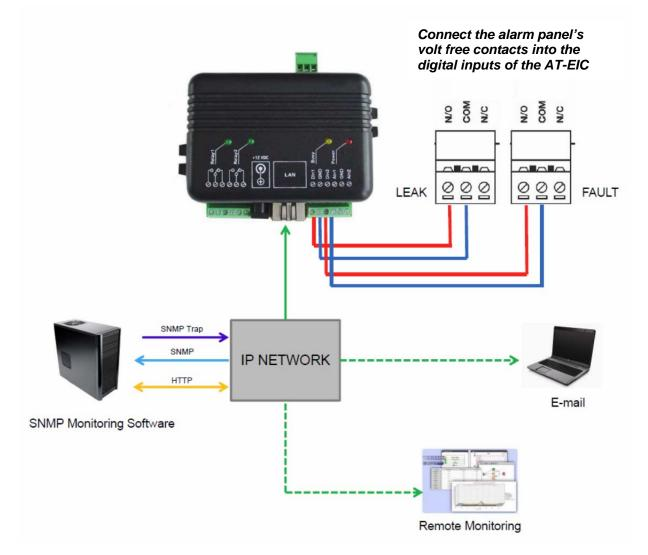
A volt free contact is connected to one of the digital input of the AT-EIC. When the contact switches, the AT-EIC can be programmed to send a message to a predefined email address or SNMP trap messages are sent if custom SNMP software is used.
